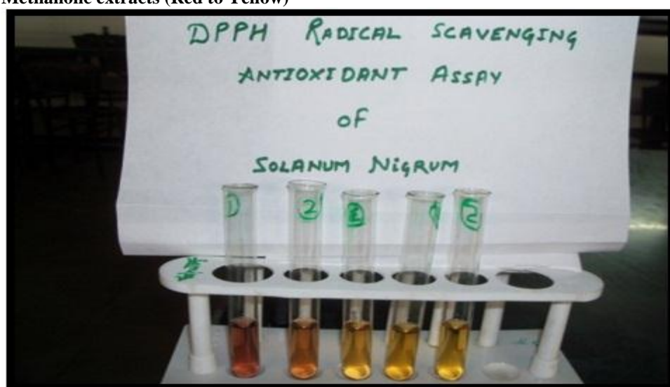
Figure 8. DPPH Radical Scavenging Antioxidant Assay Of Solanum nigrum ; colour change due to increased concentration of Methanolic extracts (Red to Yellow)
